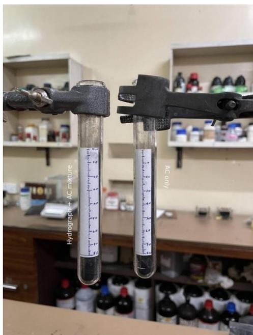
**Figure 5.** Experimental setup for observing diffusion rates of electrolyte in electrode materials.
