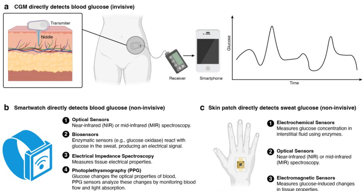
**Figure 3. Wearable devices for direct glucose monitoring.** (a) CGM systems directly measure blood glucose levels using sensors inserted beneath the skin. These systems continuously track glucose levels and transmit the data to connected devices for real-time monitoring. CGM: continuous glucose monitoring. (b) Smartwatches are equipped with sensors based on various principles to directly measure blood glucose levels. (c) Similarly, skin
