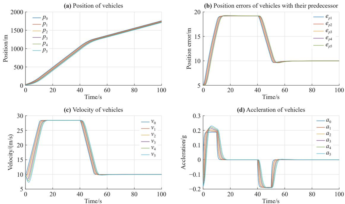
**Figure 7.** States of vehicles applying controller in [29] with headway time  $h = 0.5$  s and estimator (4). (a) Vehicles' position; (b) Vehicle's position tracking error with regard to their direct predecessor; (c) Vehicle's velocity; (d) Vehicle's acceleration.
