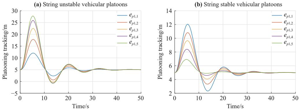
**Figure 1.** Platooning tracking errors of string unstable and string stable vehicular platoons with the safety distance being 5 m, where  $e_{p1,i}(t) = p_0(t) - p_i(t)$ . (a) String unstable vehicular platoons; (b) string stable vehicular platoons.
