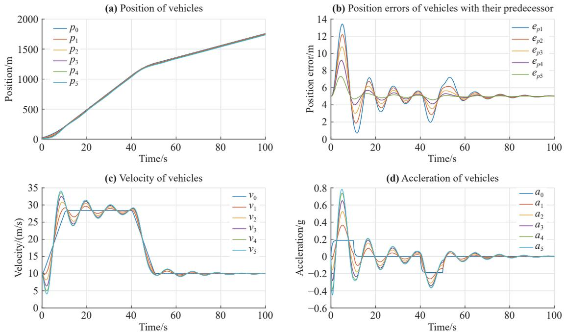
**Figure 6.** States of vehicles applying controller (6) with the headway time  $h = 0$  s and estimator (4). (a) Vehicles' position; (b) Vehicle's position tracking error with regard to their direct predecessor; (c) Vehicle's velocity; (d) Vehicle's acceleration.
