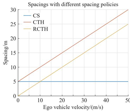
**Figure 3.** Spacing of vehicular platoons applying CS, CTH and RCTH policies with a headway time  $h = 0.5$  s when the predecessor is traveling at 10 m/s.
