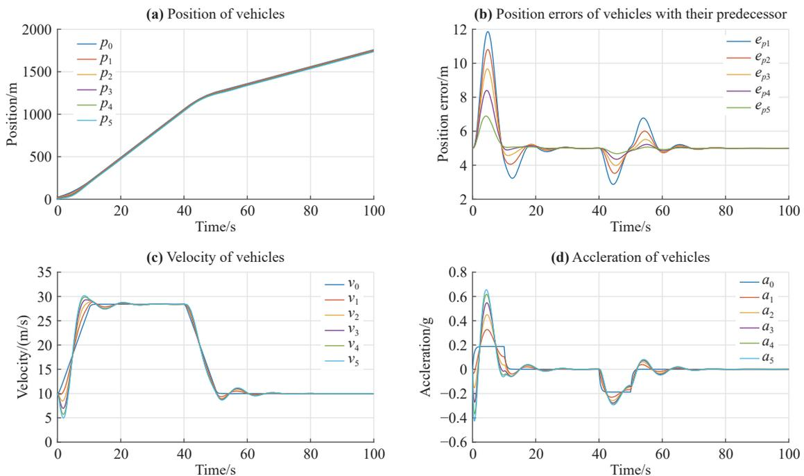
**Figure 4.** States of vehicles applying controller (6) with the headway time  $h = 0.5\text{ s}$  and estimator (4). (a) Vehicles' position; (b) Vehicle's position tracking error with regard to their direct predecessor; (c) Vehicle's velocity; (d) Vehicle's acceleration.
